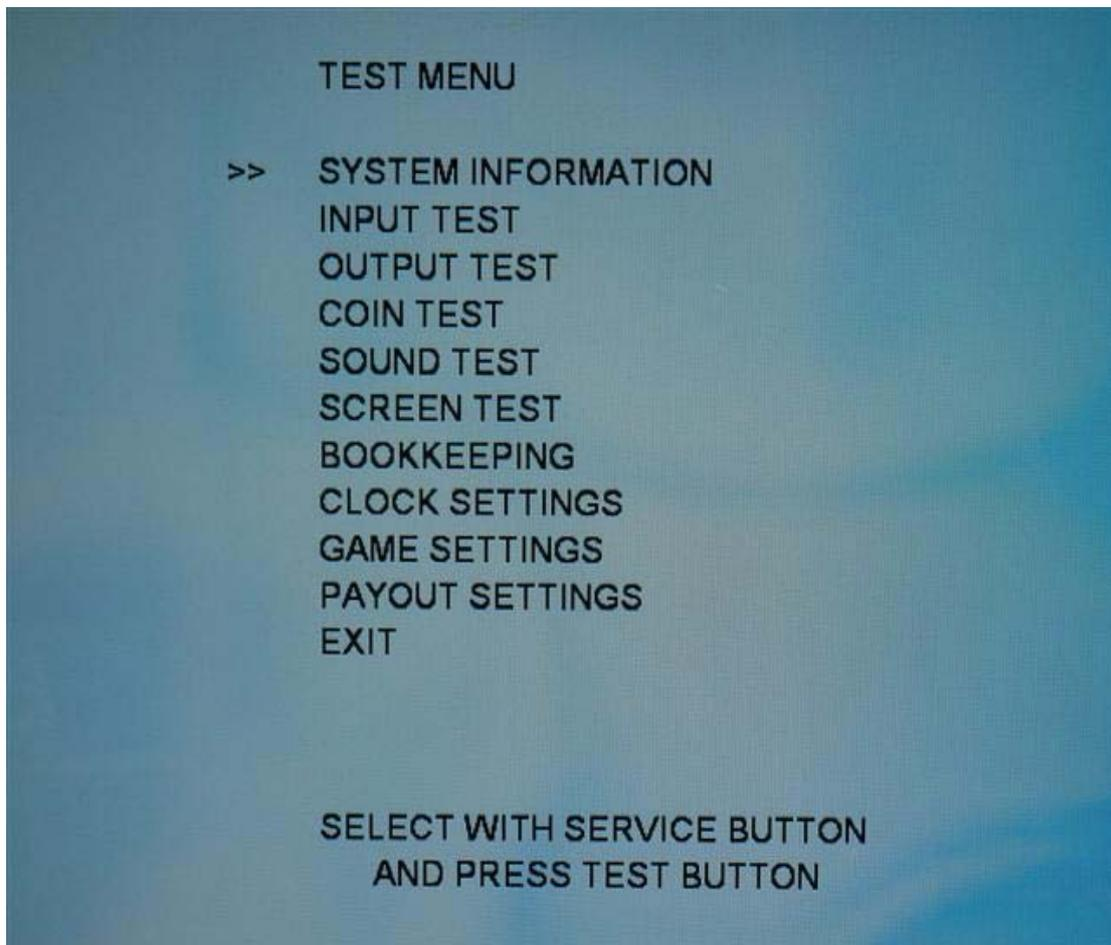
The Main Test Menu lists all of the available tests, each of which is explained in the following sections.
