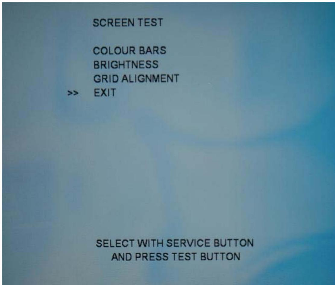
This Test is used to display various test patterns for the display screen.
