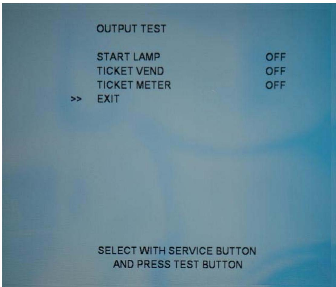
This Test is used to check System Output such as Lamps and Ticket
