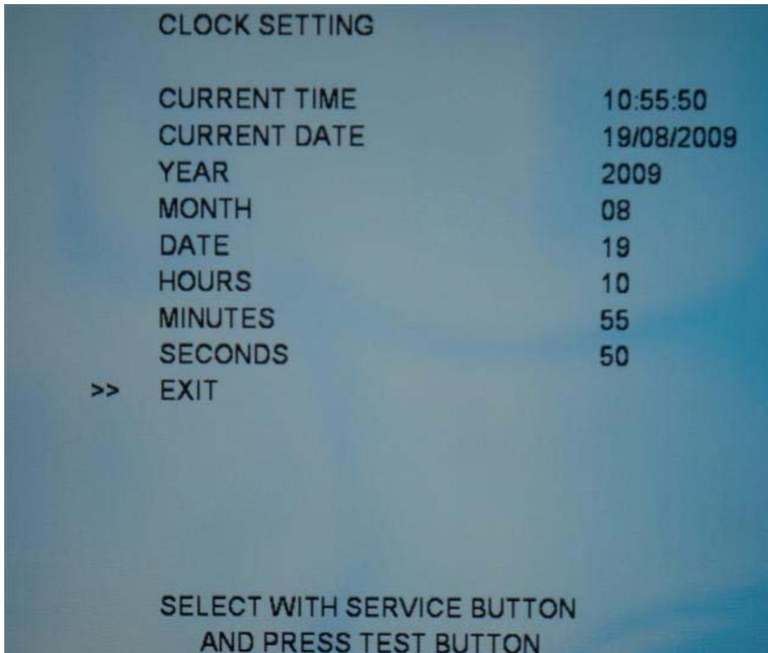
This Test is used to set the PC's real time clock facility
