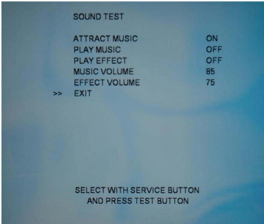
This Test is used to set Audio Levels for the Game and Test the function of the Speakers.
