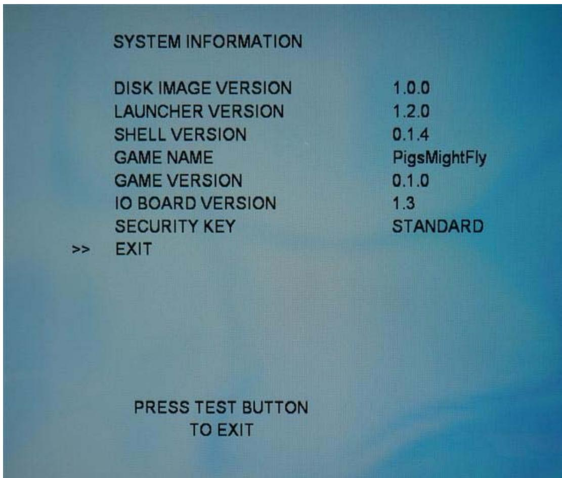
The System Information Test lists the revision numbers and names of currently installed system components.
