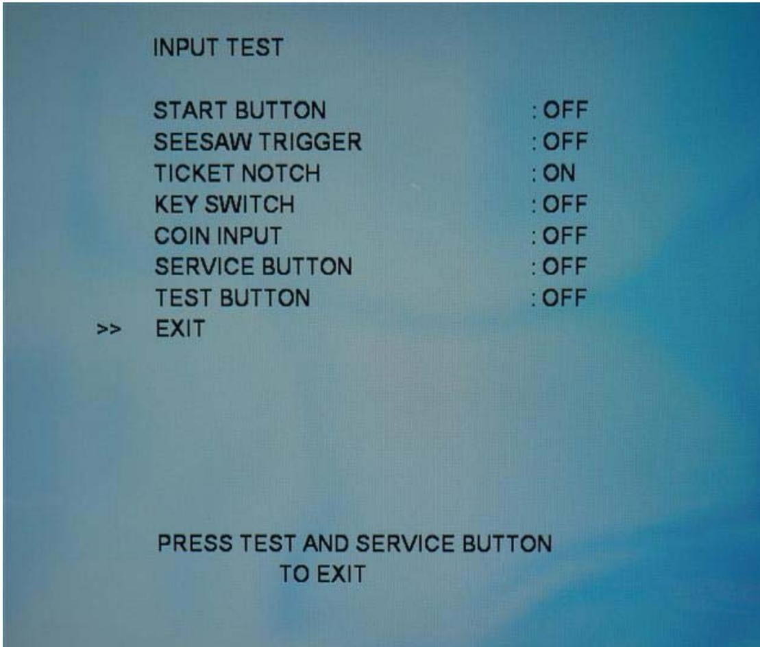
This Test is used to test the 'System Inputs' such as Seesaw Trigger and Start Button. To implement the test, Operate each device listed and check the results on screen.
